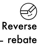
Doors with a hidden frame are also available in a reverse rebate version. This allows them to open inward while remaining flush with the wall surface from the outside.
